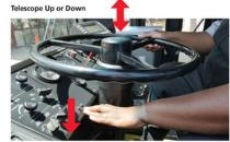
Push down on the handle located on the left side of the steering column, then adjust the height of the steering wheel as needed.
