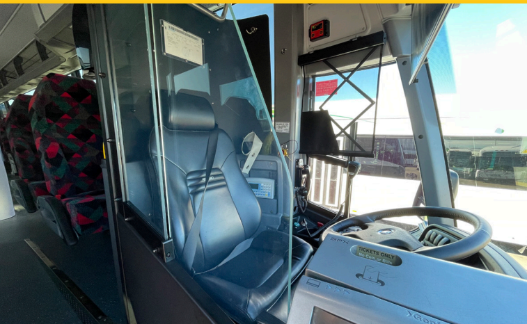
The Protective Barrier ensures that Bus Operators can focus on driving safely, minimizing the risk of accidents caused by distractions or altercations
