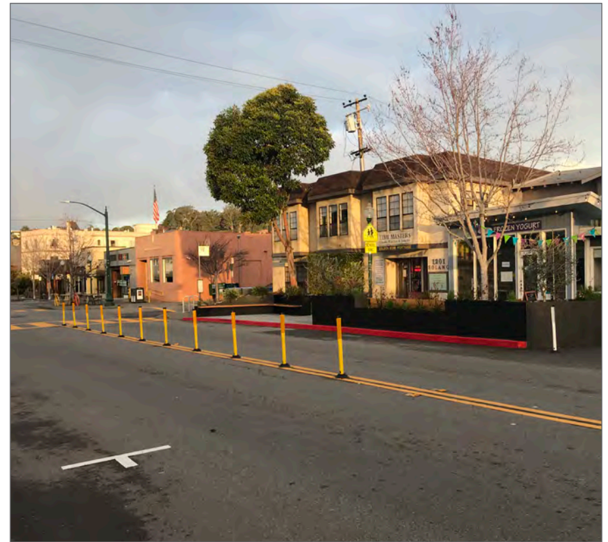
Soft-Hit Post at the Pilot Bus Parklet in Albany and Yellow Soft-Hit Posts along the centerline of the roadway
