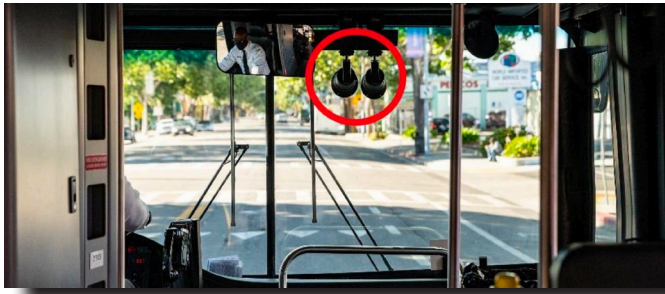
Forward-facing cameras mounted on the front windshield of Tempo coaches capture images of vehicles illegally parked in the bus only lanes.
