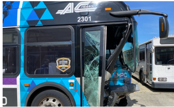
Battered and broken Coach 2301 arrived at CMF just two days after the crash, requiring replacement of the entire front section forward of the steer axle.
