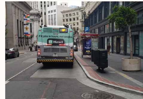
Example diagram of bus bulbs, with one stop extending into the travel lane on the left and one extending bus travel into the sidewalk zone on the right (source: CSET).
