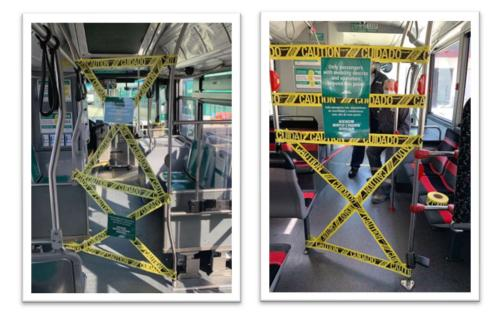
**COVID-19 Operator Shield** – In response to operator safety concerns, the maintenance team at CMF developed a shield designed to provide a layer of protection from passing riders. Pictured below is the initial design for a Gillig bus that was approved in collaboration with the AC Transit Safety Committee and ATU Local 192. Staff is working on designs for the rest of the bus fleet and is targeting to have this project completed by August 2020.
